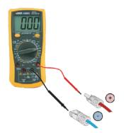
Check the positive and negative polarity of the PV strings, and connect the PV connectors to the right terminals. Serious damages to the inverter and connector over temperature may occur.
